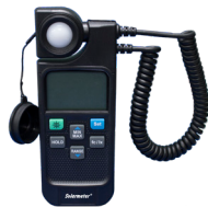
To prepare light meter for use, remove the protective cap.
